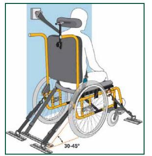
▼ It is important to use a complete WTORS to secure the wheelchair and provide the wheelchair occupant with a properly designed and tested lap/ shoulder belt system.
