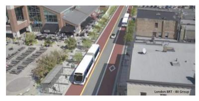
A curbside station or stop is located adjacent to the curb or parking lane of a street and is often integrated into a surrounding sidewalk.
