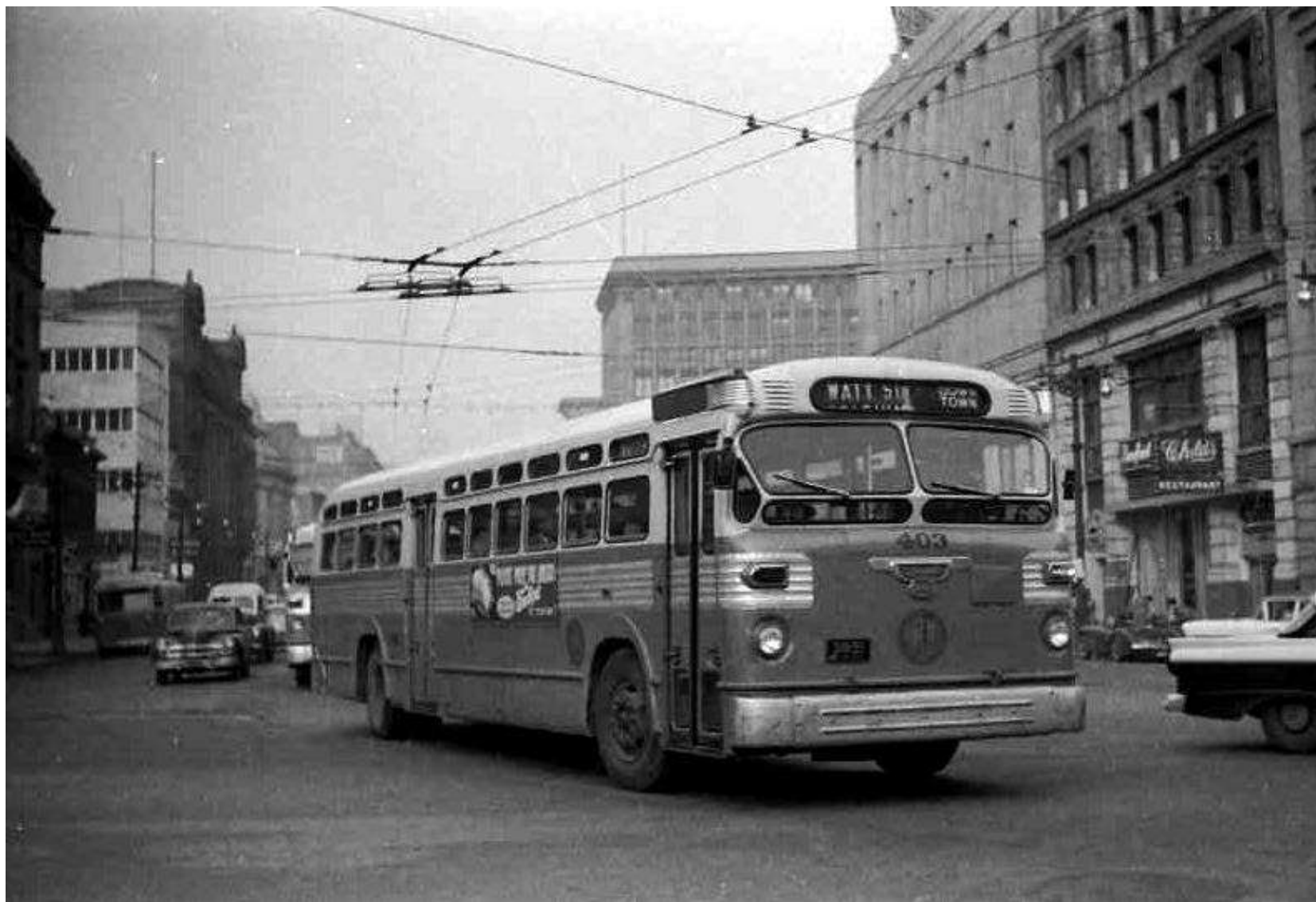
In this photograph GWTC bus 403, a 1954 Flexible-Twin Coach model FT2D-40 rounds the corner of Portage & Main destined for Watt Street. This picture was taken and provided courtesy of William A. Luke of Spokane, Washington, USA.
